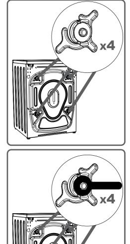
For this reason, transportation safety screws shall be loosened by being rotated in counter-clockwise using an appropriate wrench. 23
