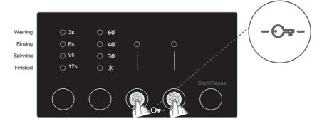
If pressed any button while child lock is active, the Additional Function Leds will blink on the display.
